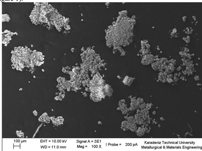
Figure 1. SEM image of a powdered ZnOTiO<sub>2</sub> NPs
