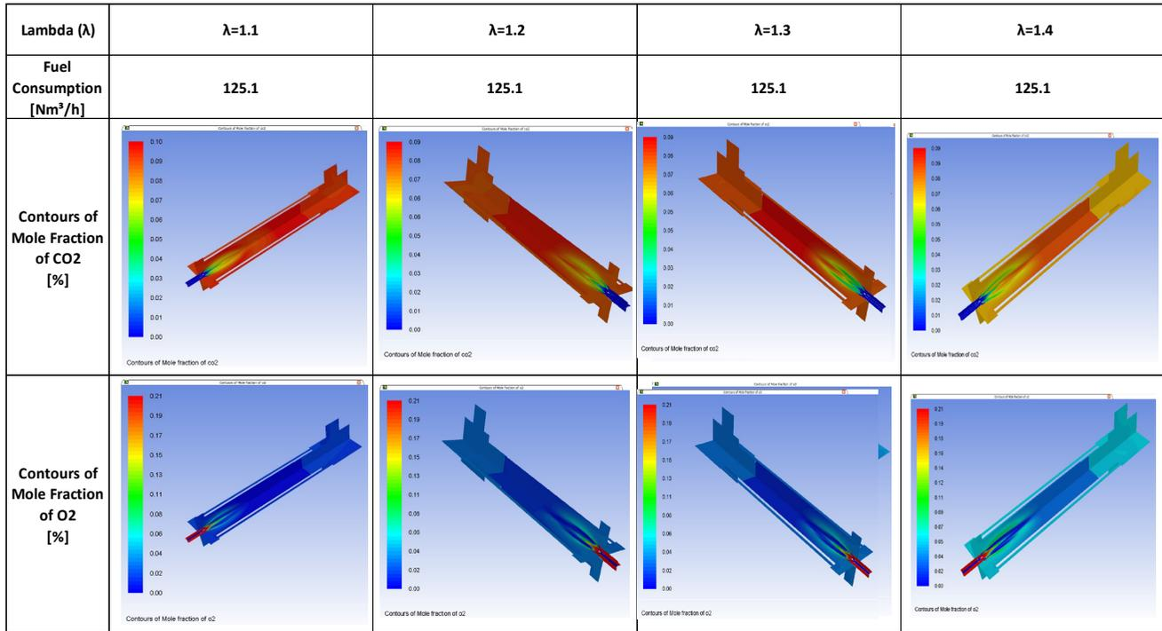
Figure 6. Contour plots of CO<sub>2</sub> and O<sub>2</sub> mole fraction distributions with varying excess air ratio.
