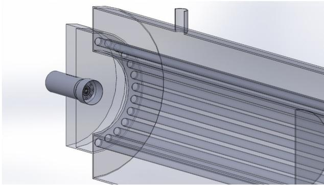
Figure 1. Simplified burner and combustion chamber geometry
