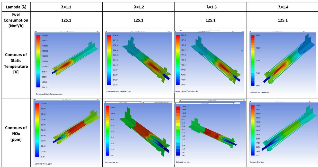
Figure 7. Contour plots of Static Temperature and NO<sub>x</sub> mole fraction distributions with varying excess air ratio.
