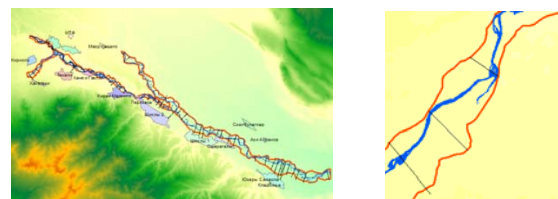
Figure 8. Creation of the cross profile of the rivers Kura, Khrami and Debed
