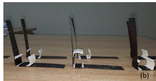
Figure 7. CFRS-C materials after being cut from plate: a) normal position b) Folded 90° on cable box.
