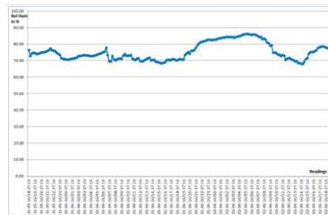
Figure 17: Relative Humidity curve for Dutta residence
