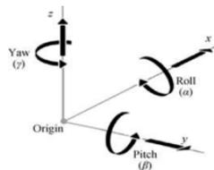
**Figure 3.** Linear and angular motions [4].
