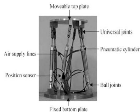
**Figure 1.** Stewart electro- pneumatic mechanism [4].
