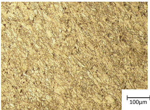
Figure 8. Piece processed through 8 stages of ECAP
