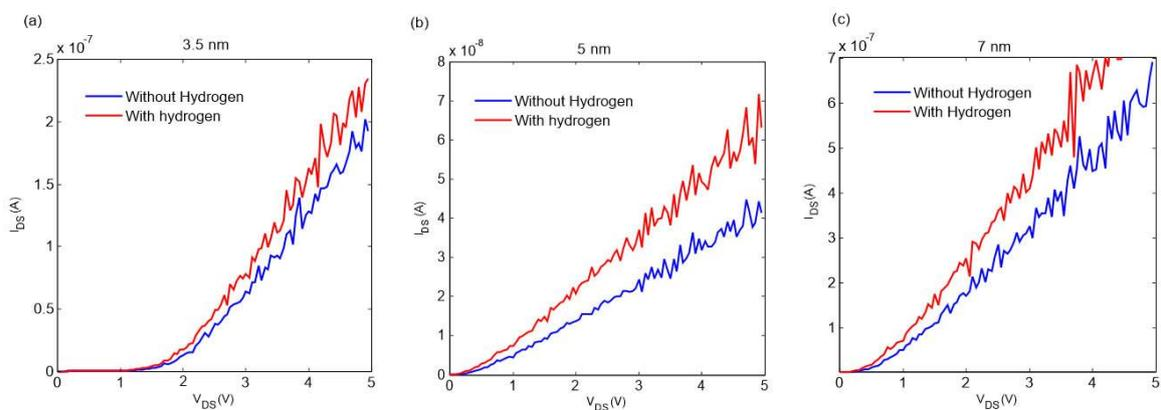
**Figure 4.** Effect of hydrogen gas on the IV characteristics of selected sections of arrays for a) 3.5 nm, b) 5 nm and c) 7 nm nano-islands.
