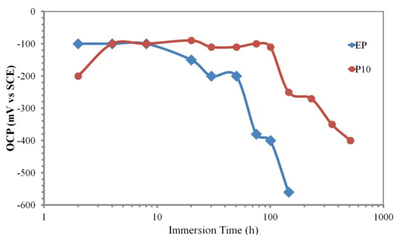
**Figure 3.** Variation of the OCP with time in 3.5% NaCl solution at 65°C for EP and P10 coatings.
