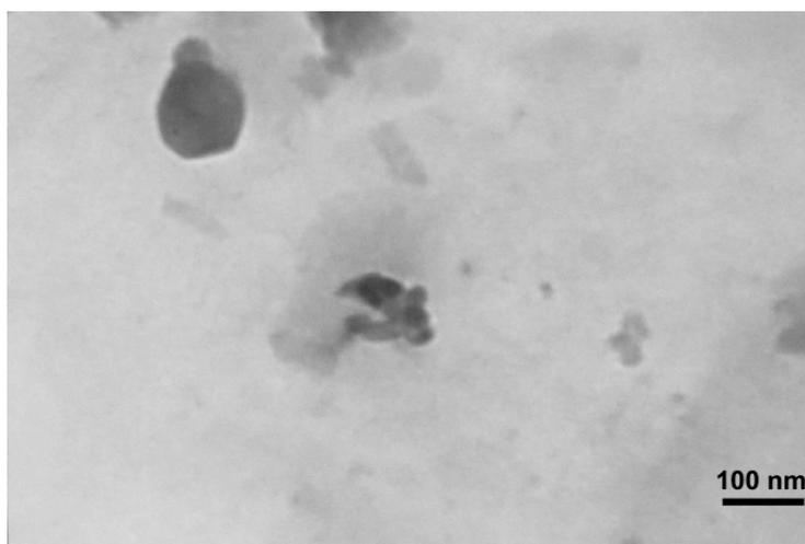
**Figure 2.** TEM micrograph of homogeneous polyaniline nanoparticles in epoxy coating.
