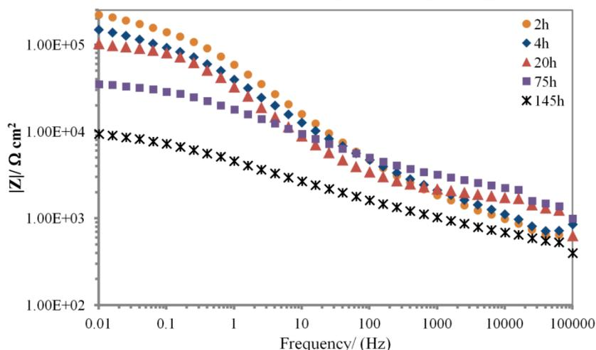
**Figure 4.** The Bode plots of the EP coating at different immersion times in 3.5% NaCl solution and 65°C.
