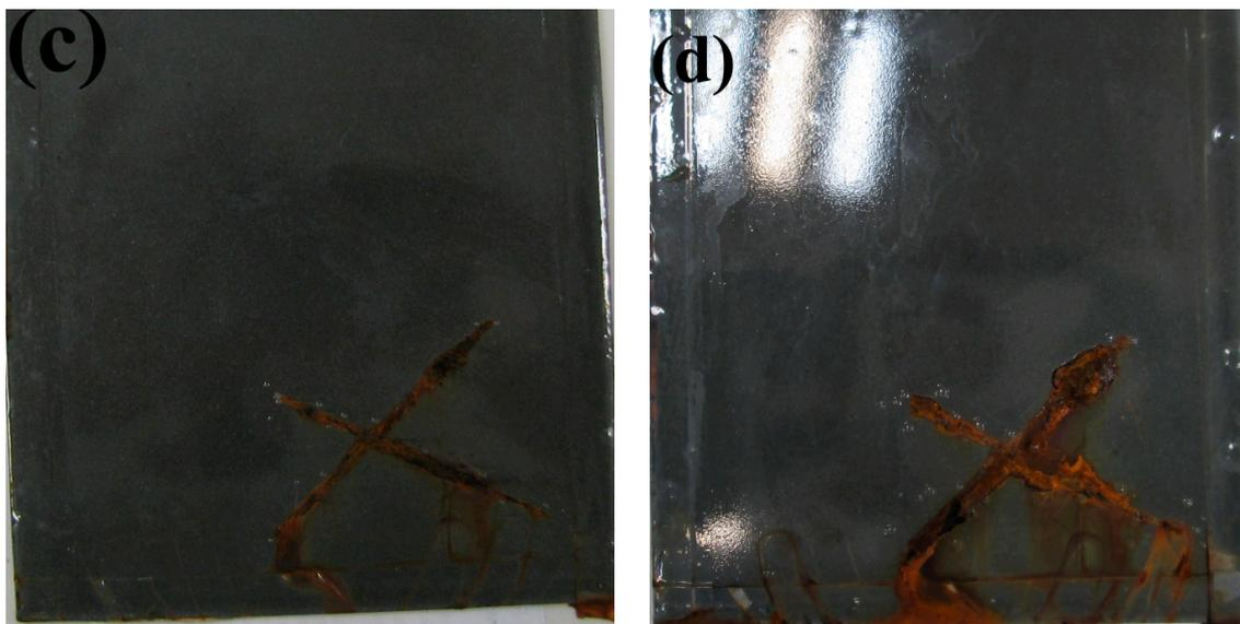
**Figure 6:** Surface appearances of the coated plates after exposing to salt spray for 168 hrs (a) EP (c) P10 and for 720 hrs (b) EP (d) P10 coatings.
