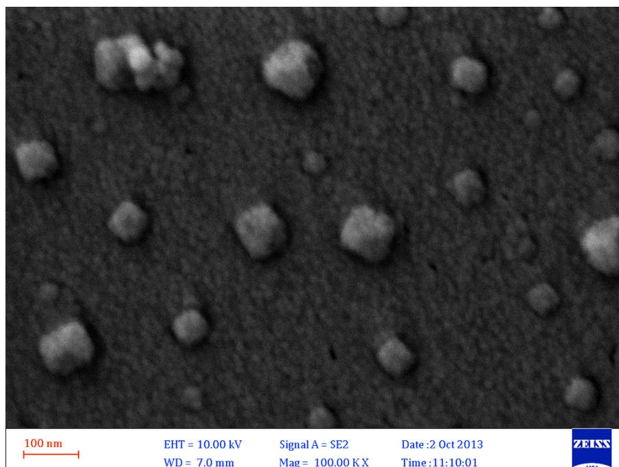
Figure 1. FESEM micrograph of synthesized polyaniline nanoparticles.
