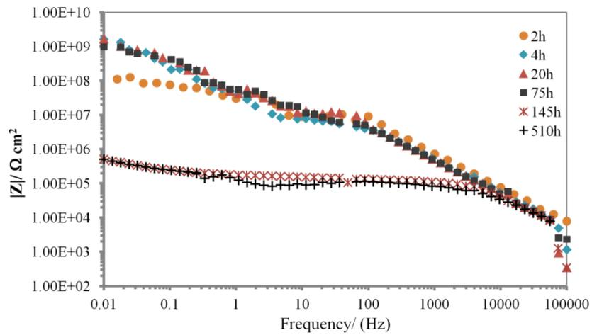
**Figure 5.** The Bode plots of the P10 coating at different immersion times in 3.5% NaCl solution and 65°C.
