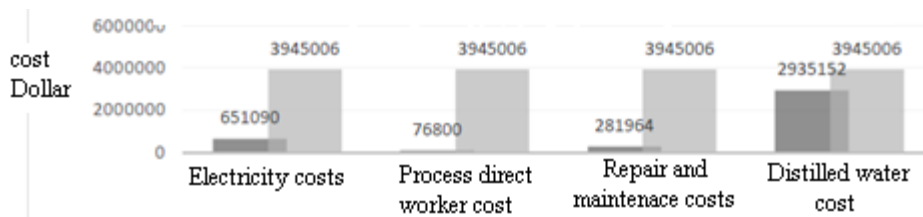
Figure 5. Operational Investment costs for fresh- water cooling tower (compensational water supply form Mobeen petrochemical Co).
