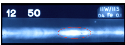
Figure 8. Excess penetration and its radiography film image
