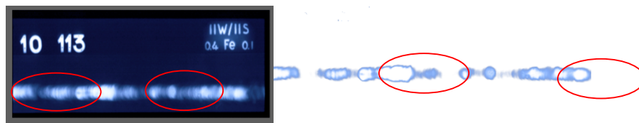
Figure 17. Radiography film image and excess weld metal cluster
