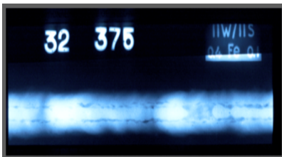
Figure 1. An example of digital radiography film image
