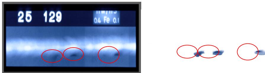
Figure 23. Radiography film image and incomplete fusion cluster
