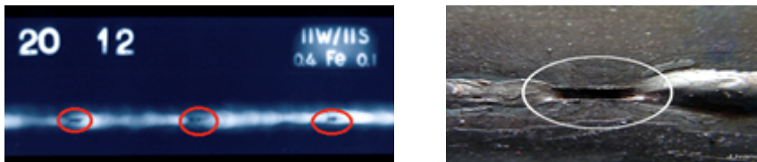
Figure 5. Incomplete penetration and related radiography film image
