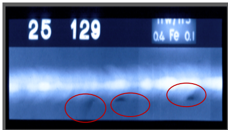
Figure 13. Incomplete fusion and radiography film image
