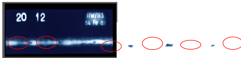
Figure 25. Radiography film image and lack of penetration cluster
