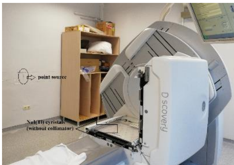
Figure 2. Gamma camera position for photopeak energy test.
