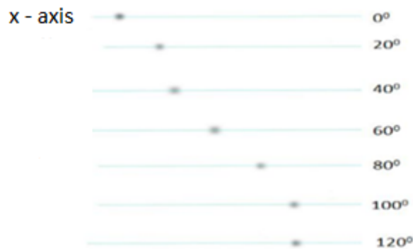
Figure 27. Point source images taken based on the varying rotation angle of the SPECT device
