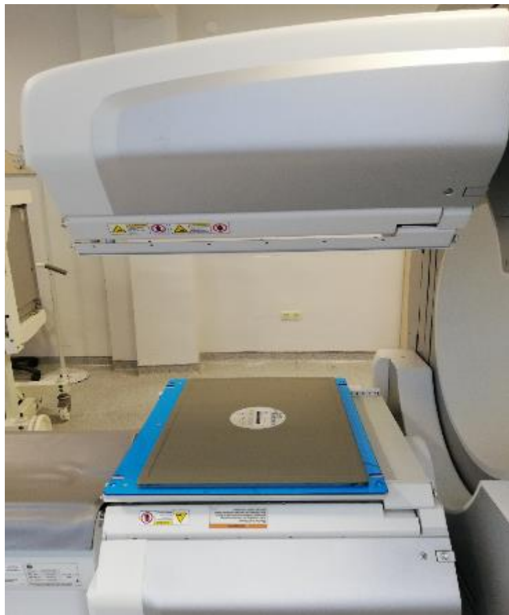
Figure 4. 4 Four- quadrant bar phantom set- up
