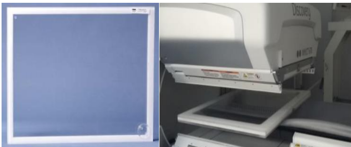
Figure 3. ^{99m}\text{Tc} Planar Sheet Source (water filled) and Extrinsic Uniformity Test Set- up
