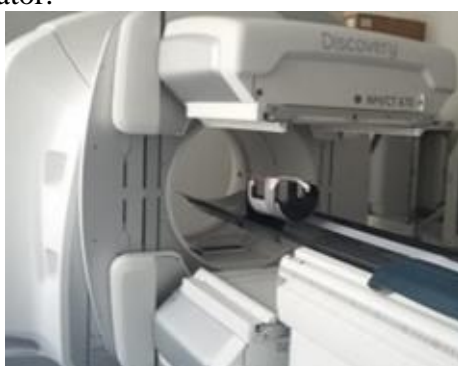
Figure 7. Placement of point source between detectors for test of Alignment of Camera with Axis of Rotation
