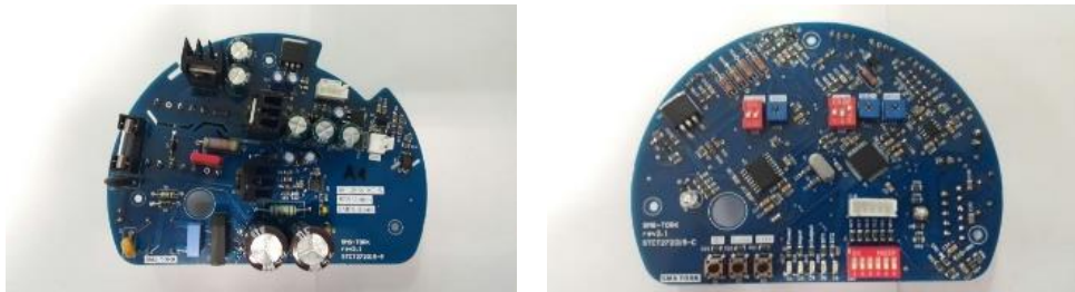
Figure 5. Designed control and SMPS boards
