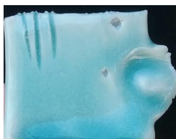
Figure 30. 1 % RIO, the barest hint of green, some sign of crazing [43]
