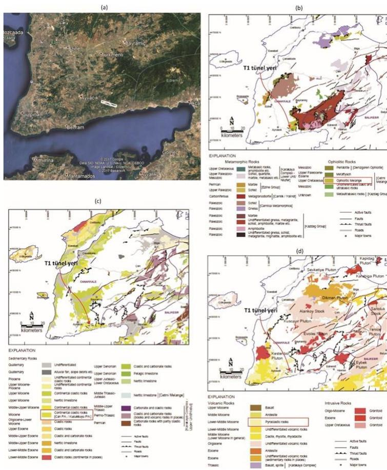
Figure 1 (a) The Location of the T1 Tunnel on the Google Earth Image, (b) The Metamorphic and Ophiolitic Rock Outcrops on the Biga Peninsula, (c) Sedimentary Rock Outcrops and (d) Volcanic Rock Outcrops (Modified from Yiğit 2012 and Öztürk & Serkendiz, 2018).
