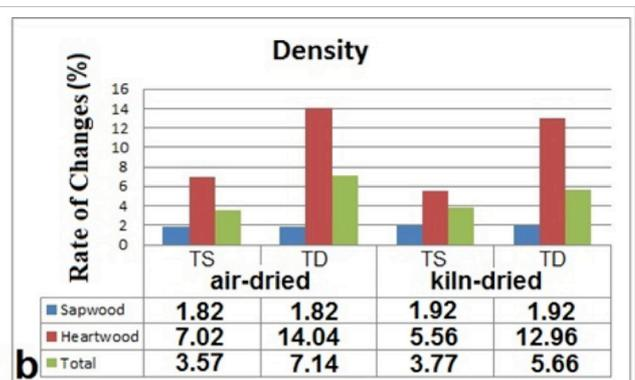
Figure 7. a, b. (a) Density values of the samples, (b) Rate of changes in densities according to reference samples
