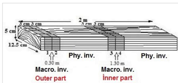
Figure 2. Cutting plan of timbers
