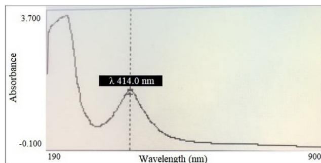
**Figure 3.** Absorption spectra of 7.5% L-PVP solution having R = 50 value.
