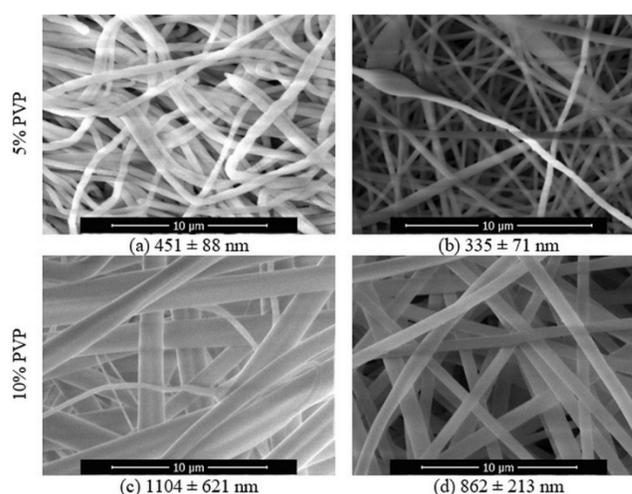
**Figure 6.** SEM images of nanofibers produced from 5% and 10% PVP solutions with compositions of (a) 1% L-PVP + 9% H-PVP, (b) 5% L-PVP + 5% H-PVP, (c) 1% L-PVP + 19% H-PVP, (d) 10% L-PVP + 10% H-PVP.
