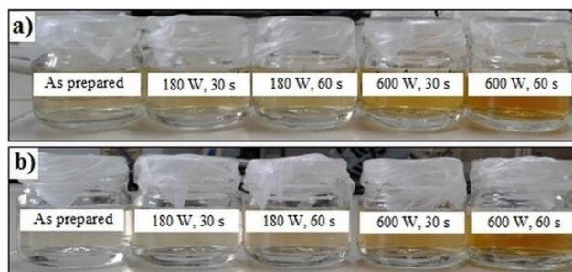
**Figure 1.** 1% L-PVP solutions containing AgNO<sub>3</sub> with the ratio of  $R = 10$  (a) and  $R = 50$  (b).
