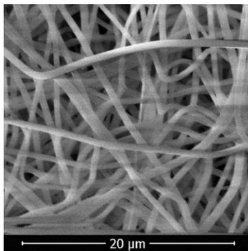
**Figure 7.** SEM images of nanofibers produced from 7.5% PVP solution.
