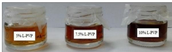
**Figure 2.** 5%, 7.5% and 10% L-PVP solutions containing AgNO<sub>3</sub> with the ratio of R = 50.
