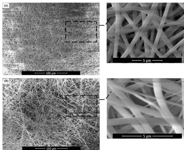
**Figure 10.** (a) neat, (b) AgNPs containing nanofibers produced from 7.5% PVP solution after thermal treatment at 200 °C for 2 h.
