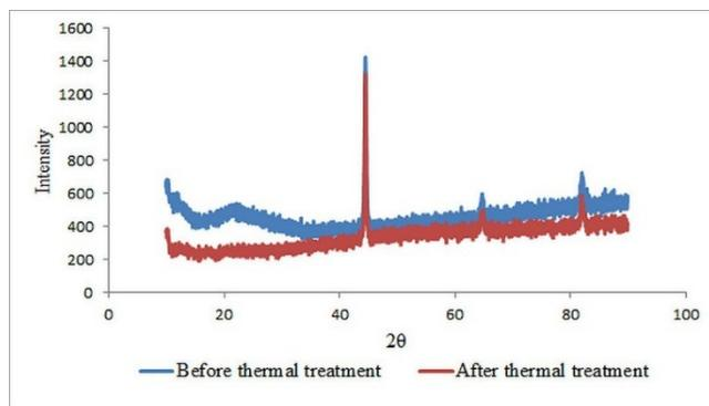
**Figure 11.** XRD patterns of AgNPs containing nanofibers produced from 7.5% PVP solutions before and after thermal treatment.
