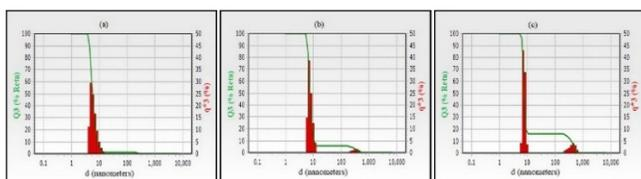
**Figure 5.** Size distributions of AgNPs synthesized in (a) 5%, (b) 7.5% and (c) 10% L-PVP solutions.
