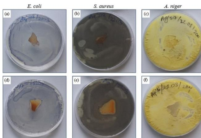
**Figure 12.** Zone of inhibition test against *E. coli*, *S. aureus* and *A. niger*. (a-c) neat nanofibers, (d-f) AgNPs containing nanofibers.
