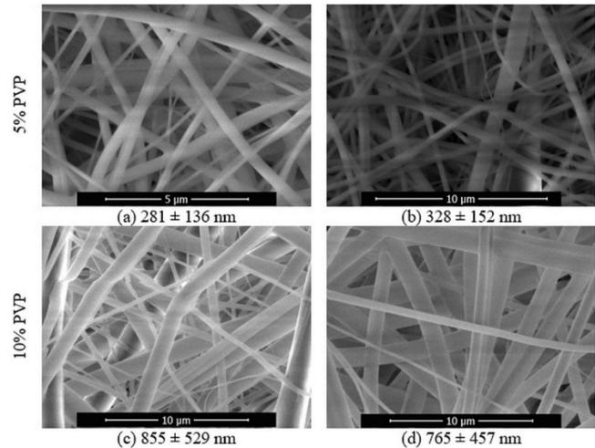
**Figure 8.** SEM images of AgNPs containing nanofibers produced from electrospinning solutions with compositions of (a) 1% L-PVP + 9% H-PVP + 1% AgNO<sub>3</sub>, (b) 5% L-PVP + 5% H-PVP + 1% AgNO<sub>3</sub>, (c) 1% L-PVP + 19% H-PVP + 0.5% AgNO<sub>3</sub>, (d) 10% L-PVP + 10% H-PVP + 1% AgNO<sub>3</sub>.
