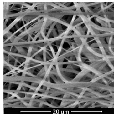
**Figure 9.** SEM images of AgNPs containing nanofibers produced from 7.5% PVP solution.
