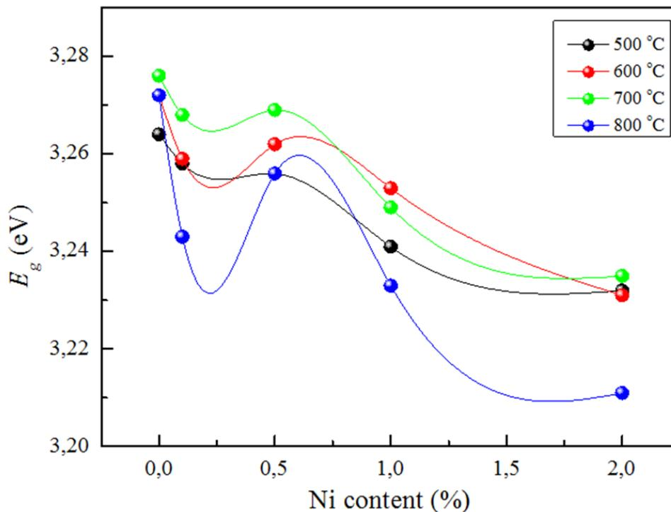
**Figure 5.** The change of the  $E_g$  with temperature
