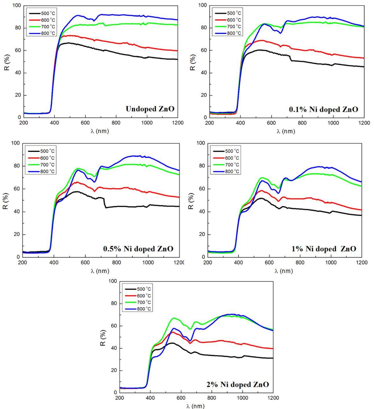
**Figure 3.** The comparison of reflectance values of samples with different sintering temperature with the same additive ratio
