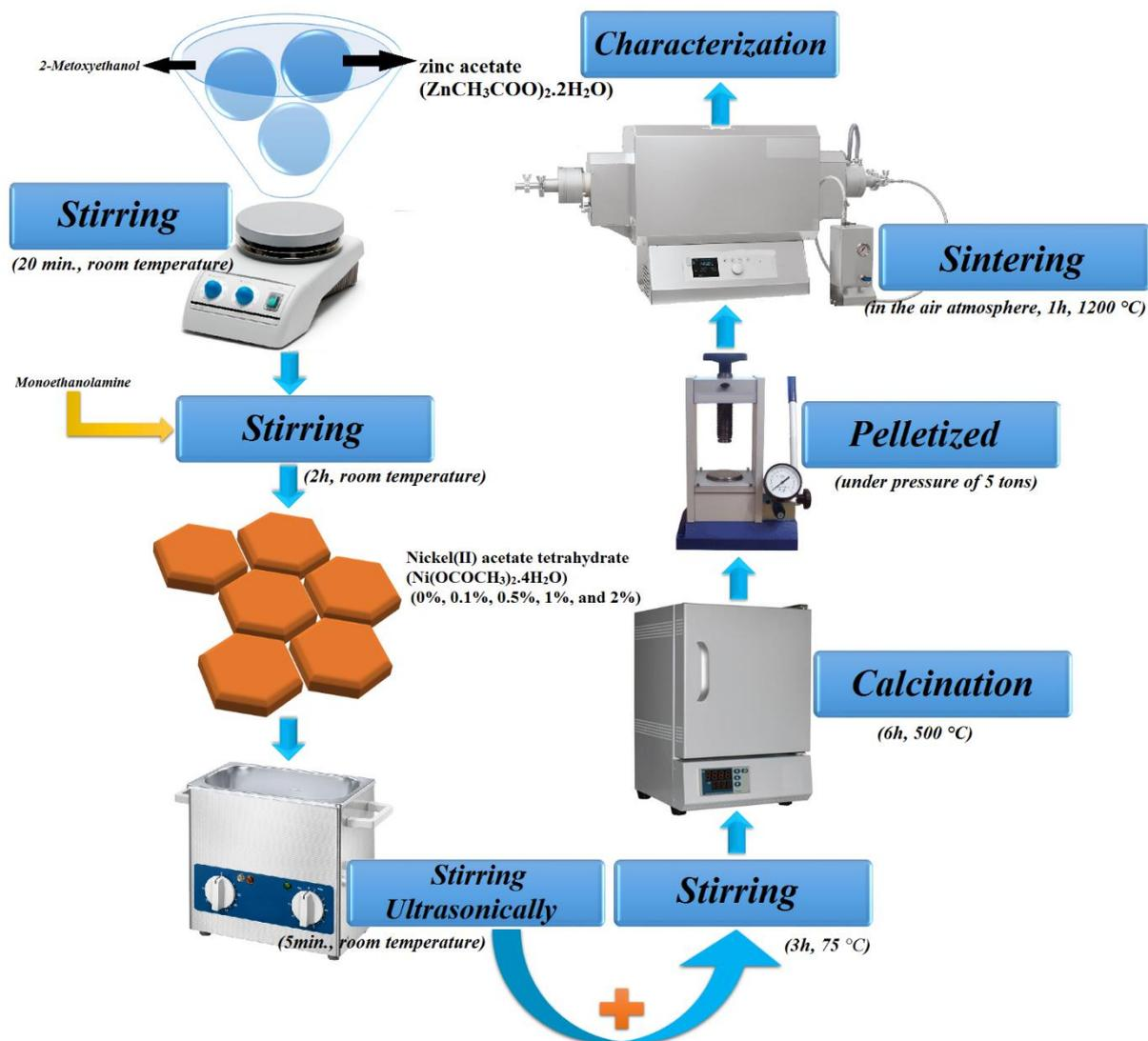
**Figure 1.** The preparation process of samples
