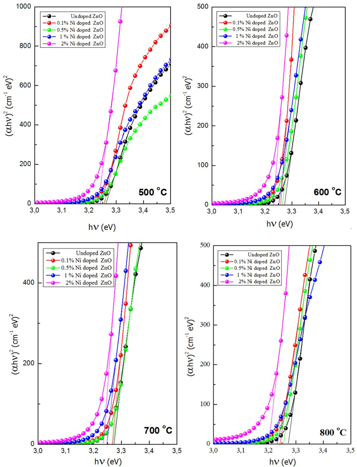
**Figure 4.** The plots of  $(\alpha h\nu)^2$  vs. the photon energy of the undoped and Ni-doped ZnO nanoceramics sintered at 500, 600, 700 and 800 °C
