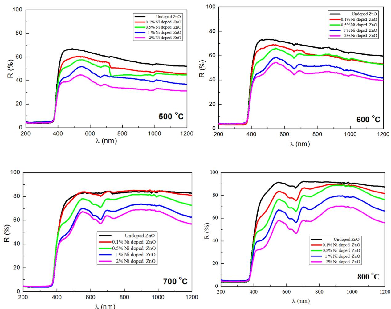
**Figure 2.** The reflectance graphs of samples sintered at 500, 600, 700 and 800 °C
