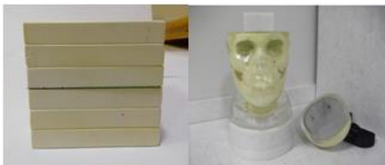
Figure 3. The positioning of the films to be irradiated in the Cyberknife phantom
