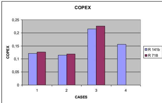
Figure 4. The comparison of COPEX values for R 141b and R 718
