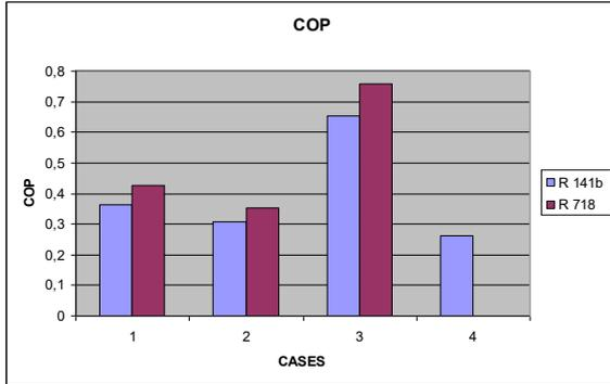
Figure 3. The comparison of COP values for R 141b and R 718
