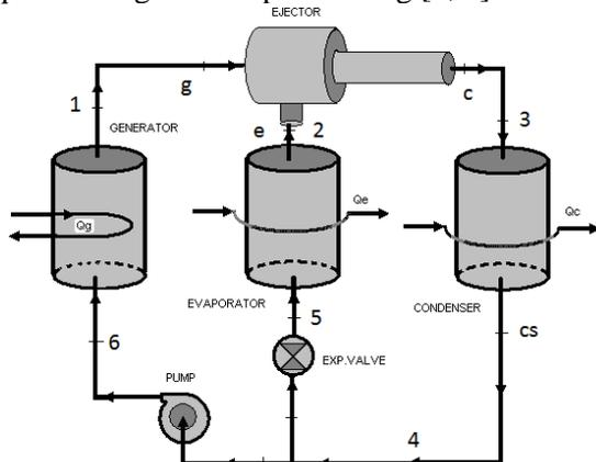
Figure 1. Schematic view of an ejector cooling system
