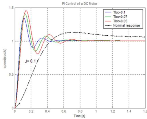
FIGURE 2. Step response with classical PI controller
