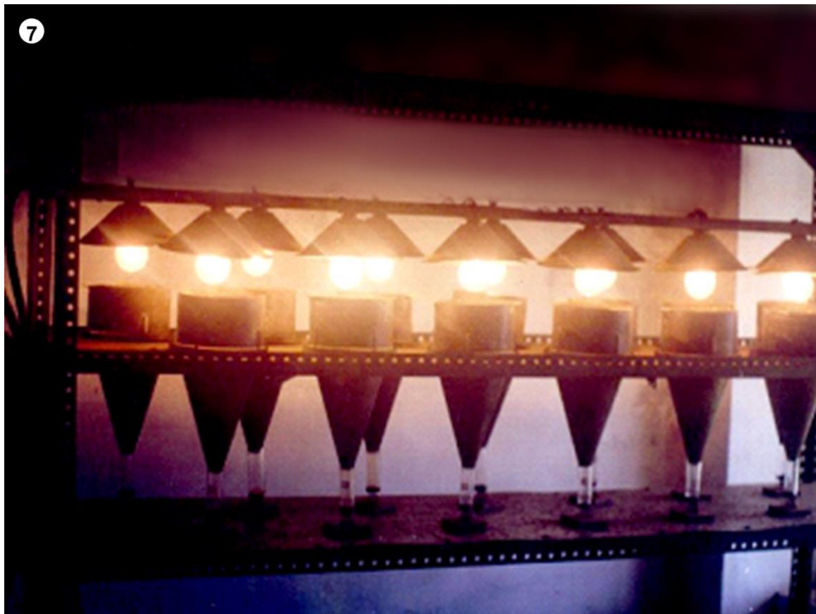
Figure 7. Open Brass Funnel Apparatus used for extraction of mites (Haq and Ramani 2002).
