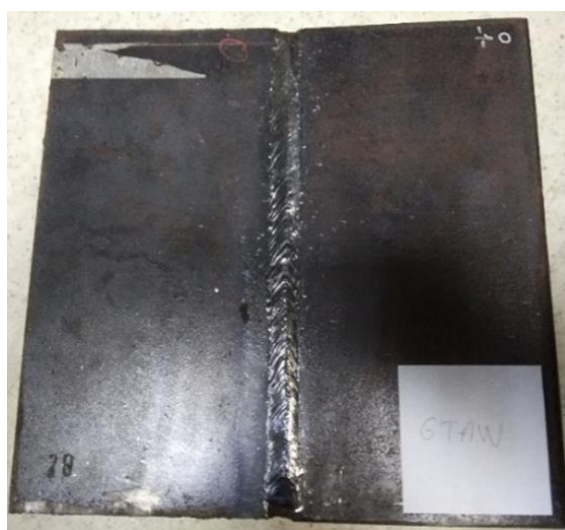
Figure 5. Welded plates with SMAW and GTAW
