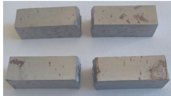
Figure 14. Test specimens after impact tests
