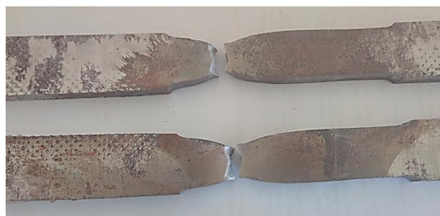
Figure 9. Test specimens after tensile tests
