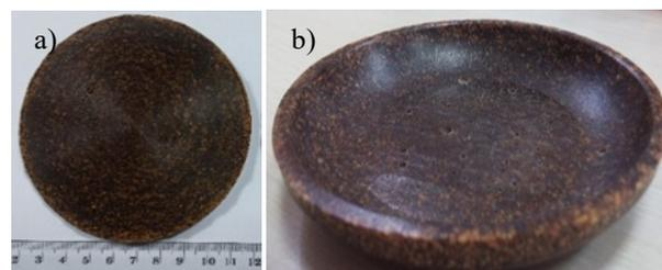
Fig. 2. Waste bio-composite applications a) teapot base b) tea plate.
