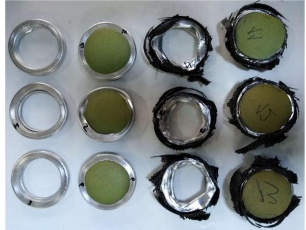
Figure 12. Specimen views after test
