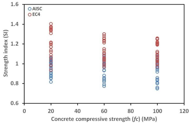
Figure 10. Effect of  $f_c$  on the Strength Index  $SI$
