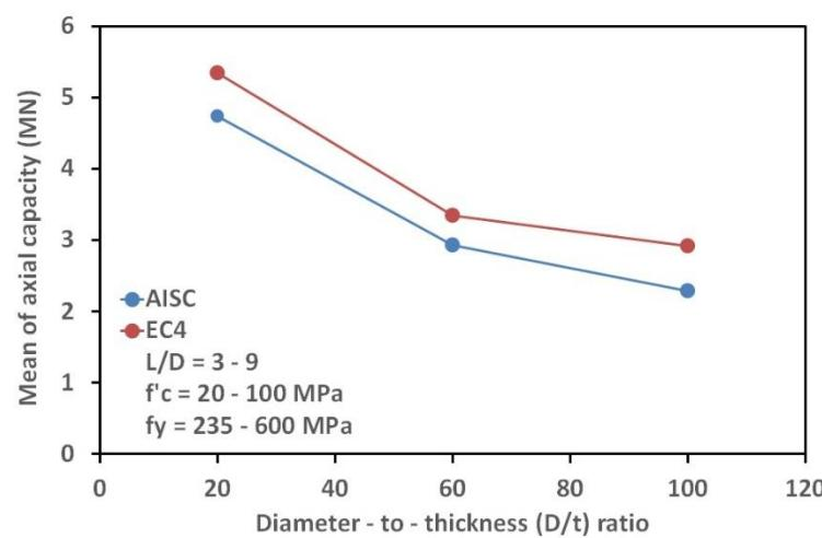
Figure 8. Mean Effect Plot of D/t Ratio
