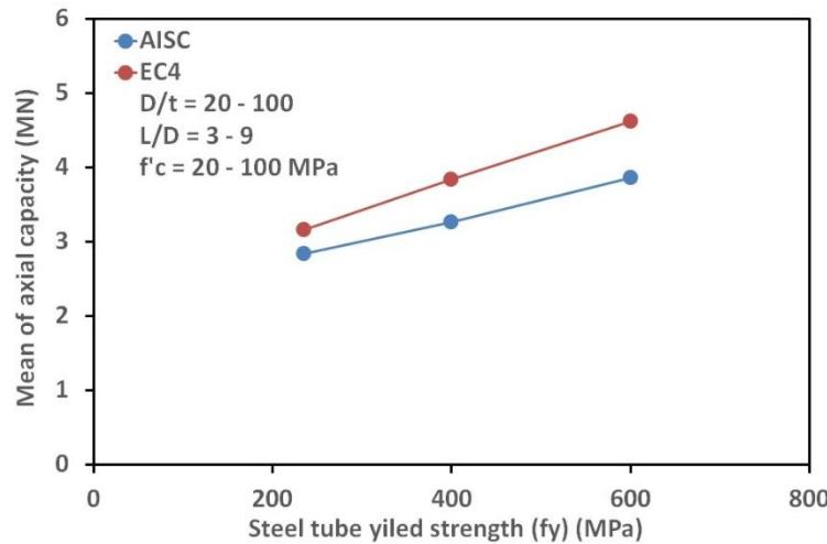
Figure 7. Effect of  $f_y$  on Axial Capacity of CFST Columns
