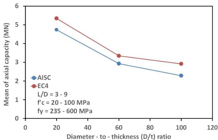
Figure 8. Mean Effect Plot of  $D/t$  Ratio
