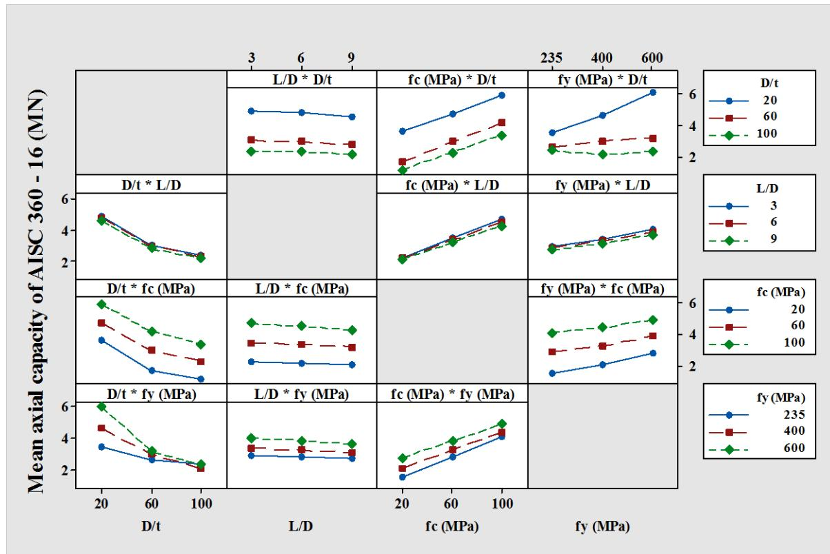
Figure 4. Interaction Plot of AISC 360 – 16 Design Code
