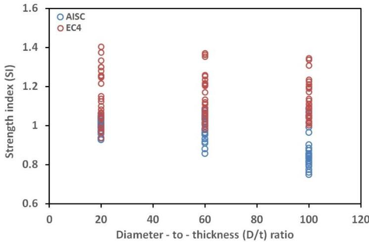
Figure 12. Effect of D/t Ratio on the Strength Index SI
