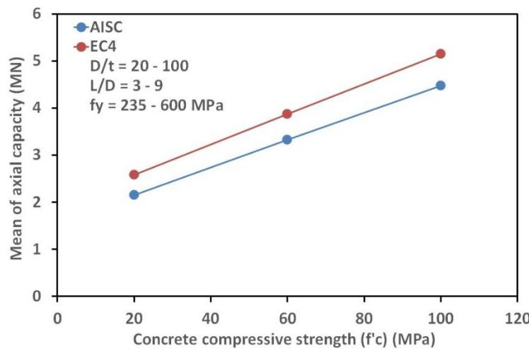
Figure 6. Effect of  $f_c$  on Axial Capacity of CFST Columns
