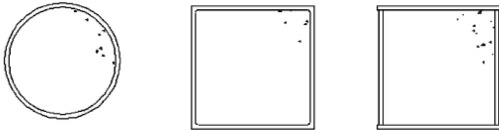
Figure 1b. Concrete-Filled Composite Columns
