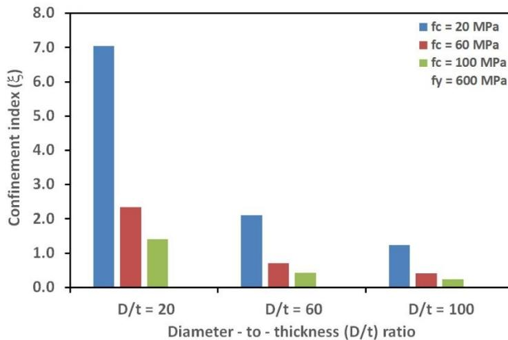
Figure 16. D/t Ratio Versus the Confinement Index  $\xi$ ,  $f_y = 600 \text{ MPa}$
