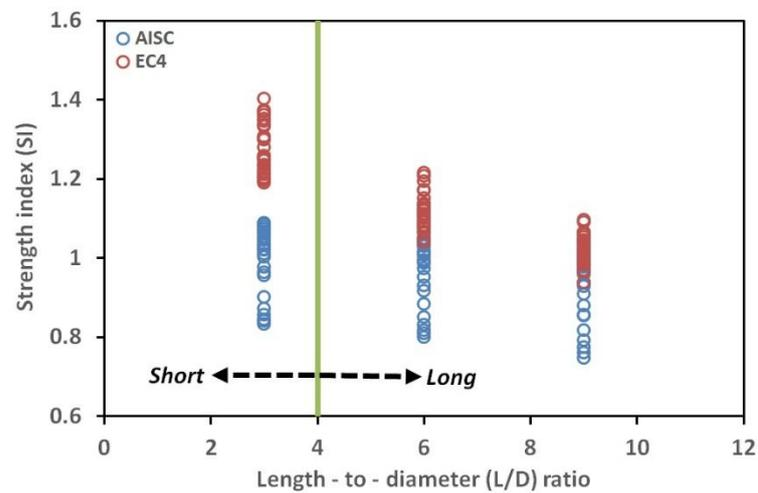
Figure 13. Effect of L/D ratio on the Strength Index  $SI$
