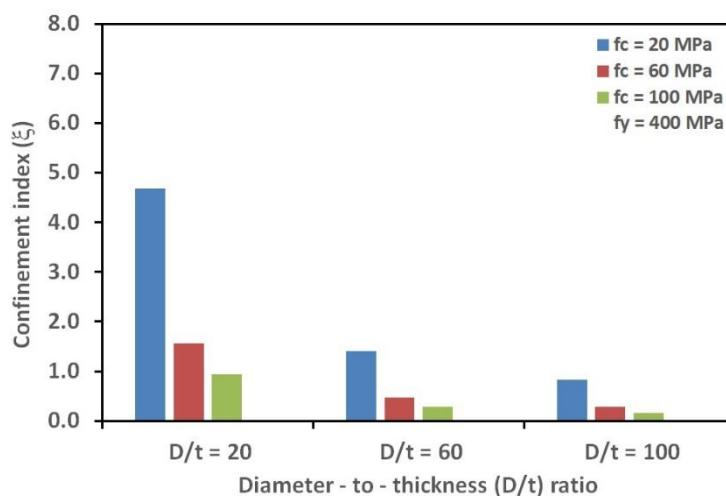
Figure 15. D/t Ratio Versus the Confinement Index  $\xi$ ,  $f_y = 400 \text{ MPa}$
