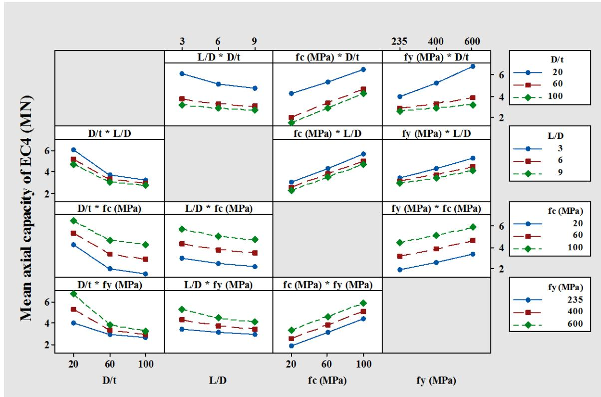
Figure 5. Interaction Plot of EC4 Design Code
