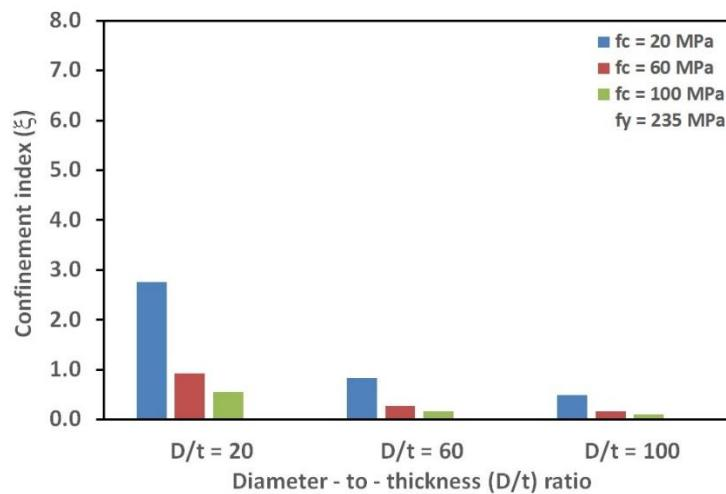
Figure 14. D/t Ratio Versus the Confinement Index  $\xi$ ,  $f_y = 235 \text{ MPa}$
