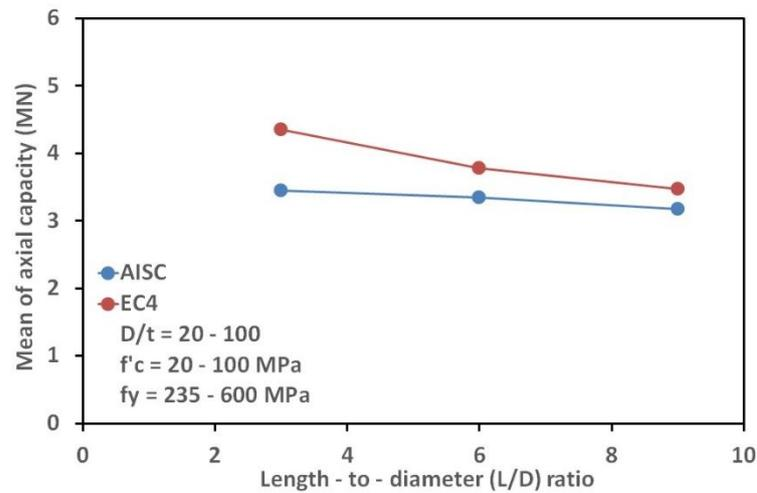
Figure 9. Mean Effect Plot of L/D Ratio
