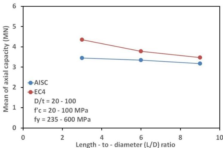
Figure 9. Mean Effect Plot of L/D Ratio
