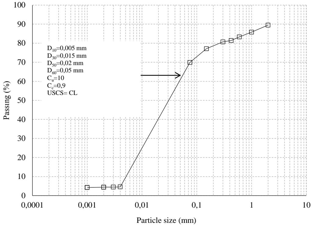
Fig. 2. Particle size distributions for the clay used the experimental study
