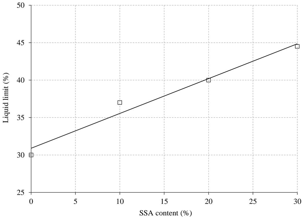
Fig 4. Liquid limit of clay with various SSA content
