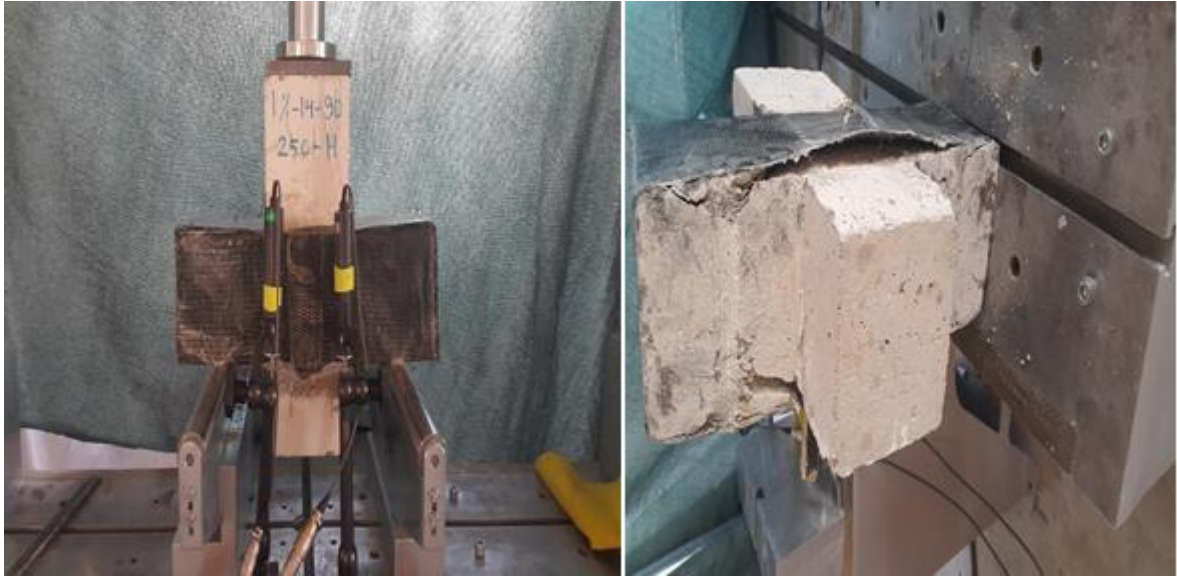
Figure 5. Specimen with De-bonding failure
