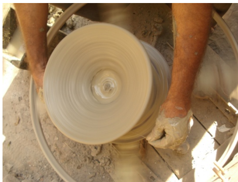
Figure 11: A lid is separated from the wheel by using soot
