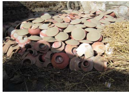
Figure 22: Filling of gaps with dry straws and potsherds
