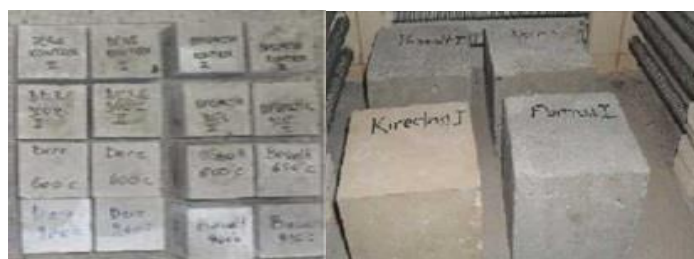
Figure 2. Cubic concrete samples produced using four different types of aggregates in two sizes (100x100x100 mm & 150x150x150 mm)
