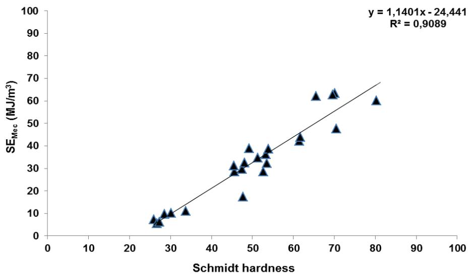
Figure 5. Prediction of  $SE_{Mec}$  using P-wave velocity (a) and Schmidt hardness (b) values of rocks
