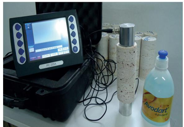
Figure 1. Sound velocity test equipment
