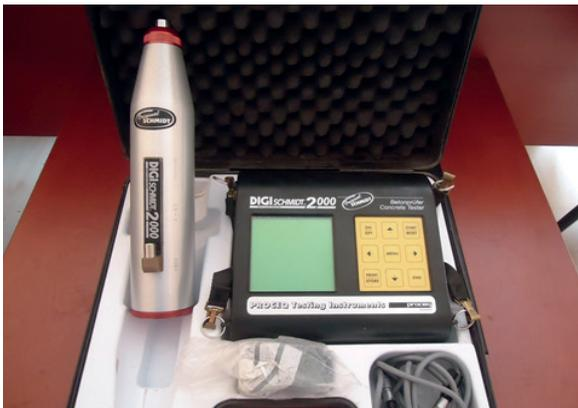
Figure 2. Schmidt hammer hardness test equipment
