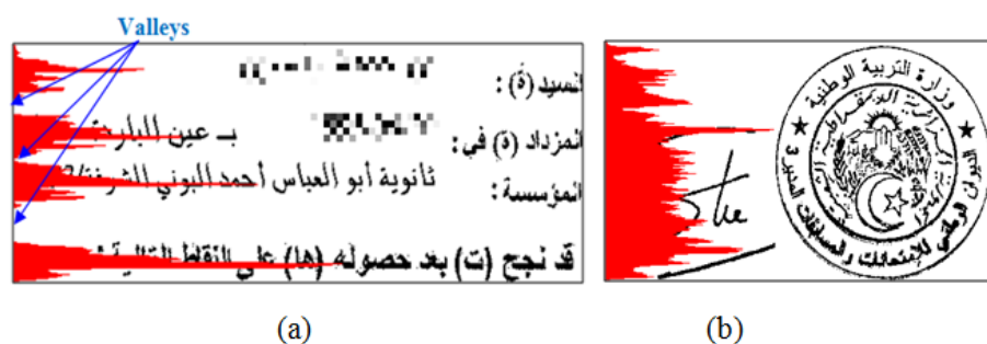
Fig. 11. Horizontal projection profile, (a) of a textual block, (b) of a non-textual block.
