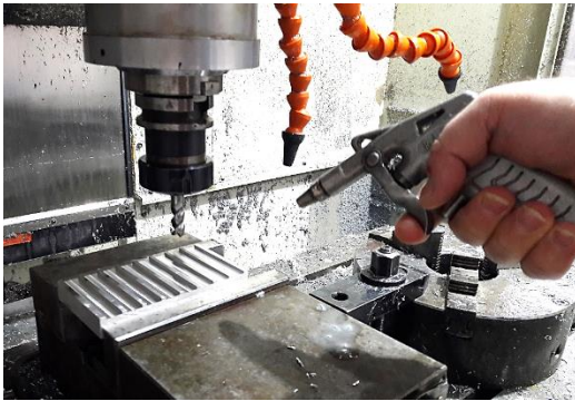
Figure 4. Milling process by cooling air
