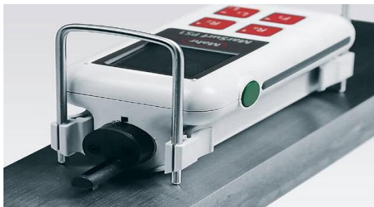
Figure 5. The Mahr-Marsurf PS1 model desktop surface roughness tester
