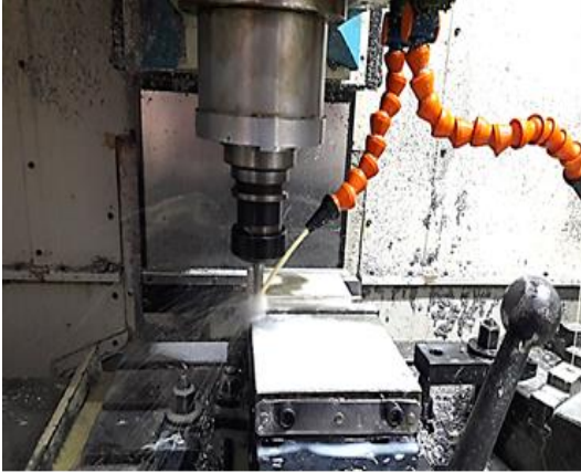
Figure 3. Milling process by cooling liquid
