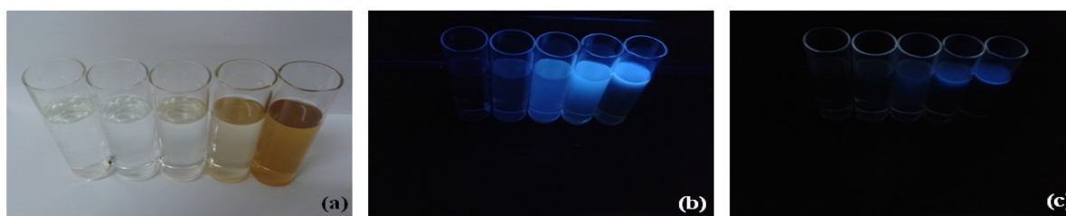
Figure 8. Left to right, distilled water ( 1.10^{-3} g, 1.10^{-2} g, 1.10^{-1} g and 1 g of P3 in 100 mL of distilled water) pictured under visible illumination (a), UV-A lamp (360 nm) (b); UV-C lamp (254 nm) (c).
