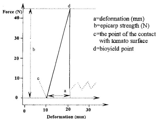
Figure 2. Typical force/deformation curve obtained during penetration or suppression of individual tomato during destructive firmness evaluation.
