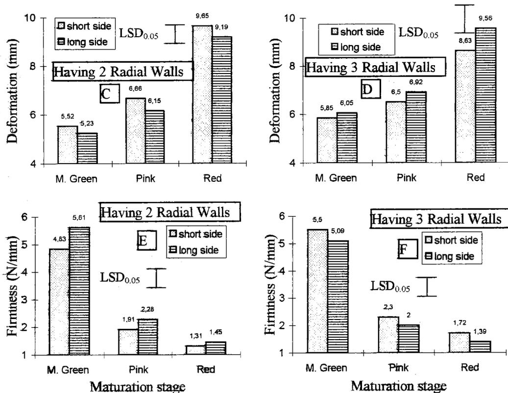
Figure 3. Epicarp strength, deformation and firmness values obtained from destructive firmness measurement of tomatoes having 2 or 3 radial walls.
