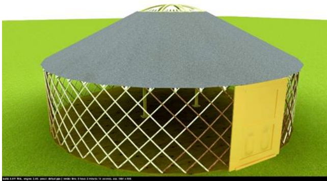
Figure 8. “Deever” (Roof covering) After building up the GER structure, the felt is put above the rafters like shown in the figure 3.
