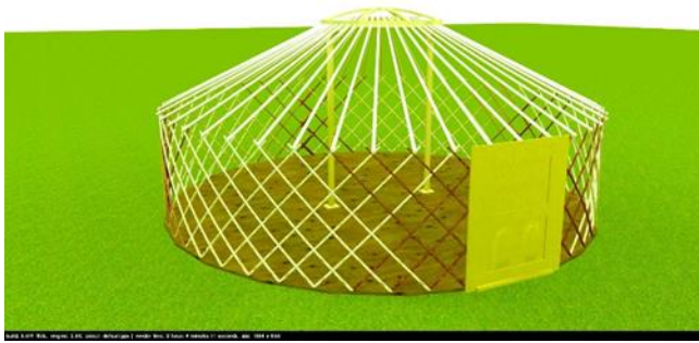
Figure 7. “Khaalga” (Door) Mongolian GER door directs to the south traditionally. It receives 6 rafters on it.
