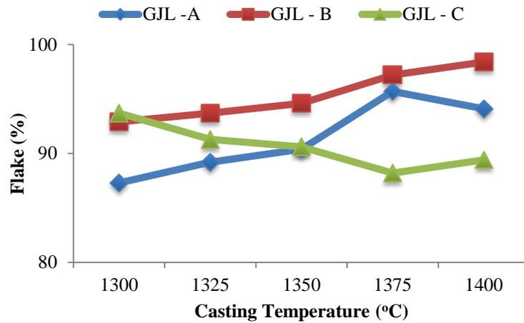
Figure 1. Change in flux amount of flake graphite cast iron materials depending on casting temperature
