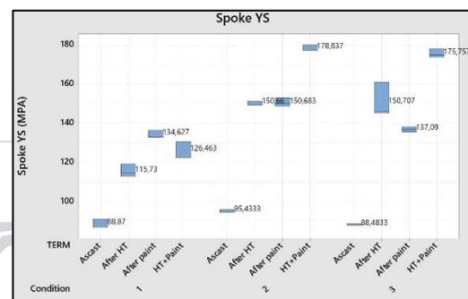
Figure 5. (a) YS of Tensile Test Specimen (Permanent Mold)
