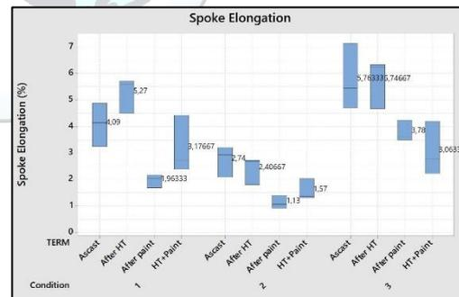
Figure 6. (a) Elongation of Tensile Test Specimen (Permanent Mold)
