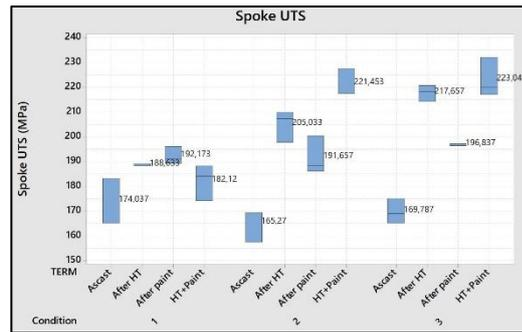
Figure 4. (a) UTS of Tensile Test Specimen (Permanent Mold)
