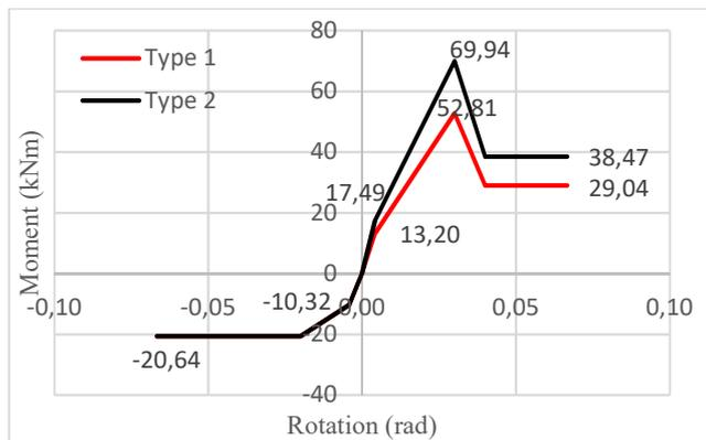
Figure 7 Moment-rotation behavior of the shear tab connections
