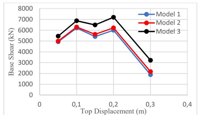
Figure 13 Base shear capacities at the target displacements
