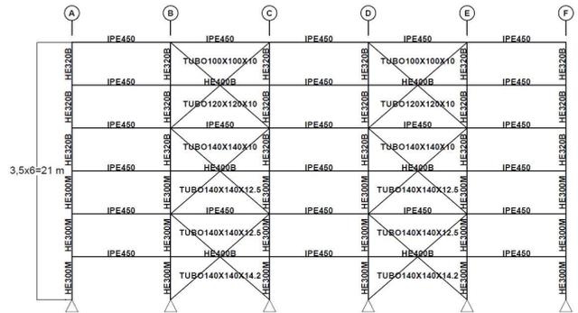
Figure 4 Elevation of the exterior frames (x direction)
