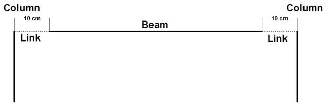
Figure 10 Modeling of nonlinear elastic link elements
