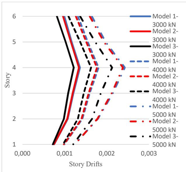
Figure 14 Story drifts under same base shear forces (a)
