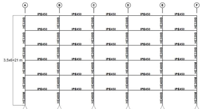
Figure 5 Elevation of the interior frames (x direction)
