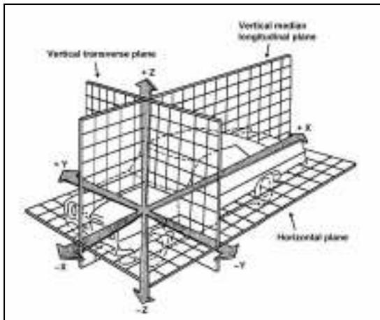
Figure 5. Vertical transverse and median longitudinal plane according to ECE R 29 [2].
