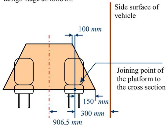
Figure 4. Dimensions of the platform of the residual space [16].
