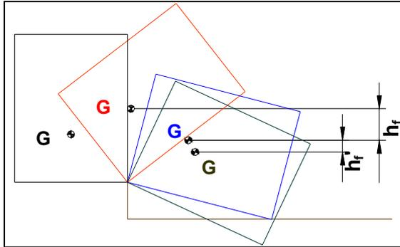
Figure 7. Course of centre of gravity of the designed bus section during the roll-over test [16].
