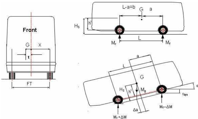
Figure 6. Characteristic distances in transverse and longitudinal bus section as well as forces acting on bus in angle of  $\alpha$  [16].
