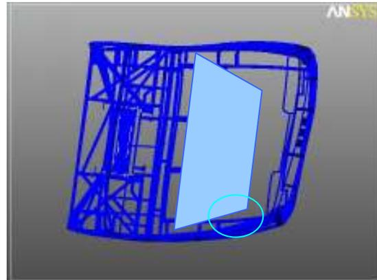
Figure 13. “Residual space” after roll-over test.
