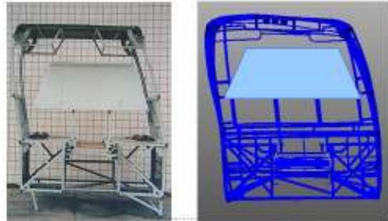
Figure 14. Comparison of the test results to the one of the FEA.
