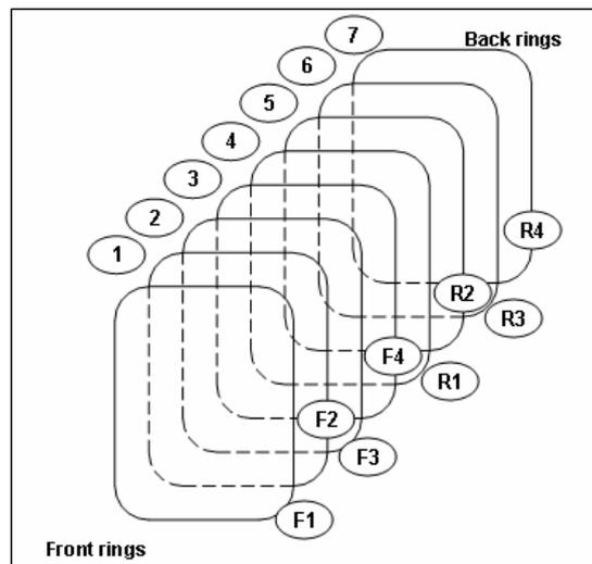
Figure 10. Representative closed rings of the bus superstructure [16].
