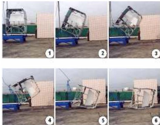
Figure 9. Roll-over test [16].
