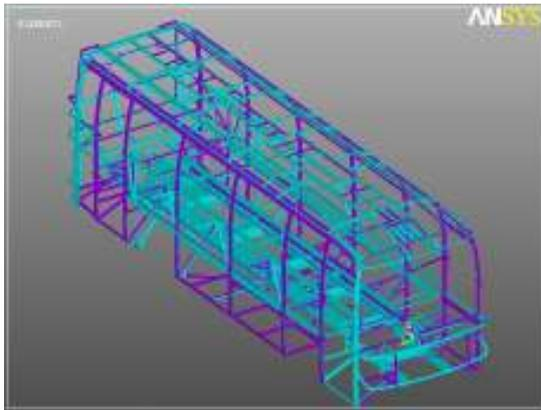
Figure 11. Model of the designed bus superstructure without sheet metal.
