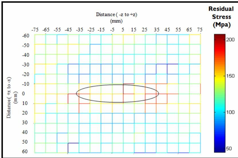
Figure 7. Total residual stress distribution throughout the welded plate
