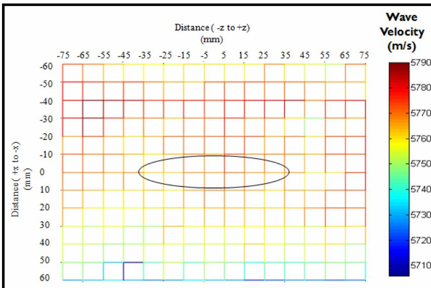
Figure 4. Ultrasonic wave velocity distribution in unwelded sample
