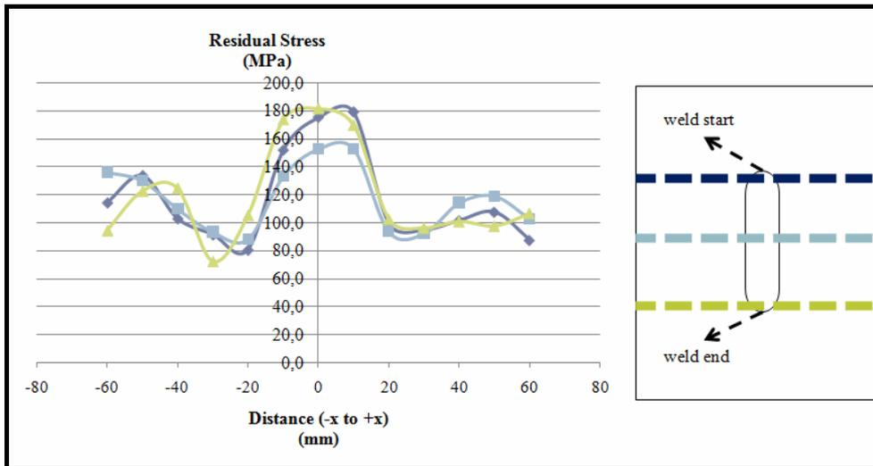
Figure 8. Total residual stress distribution through the transversal direction
