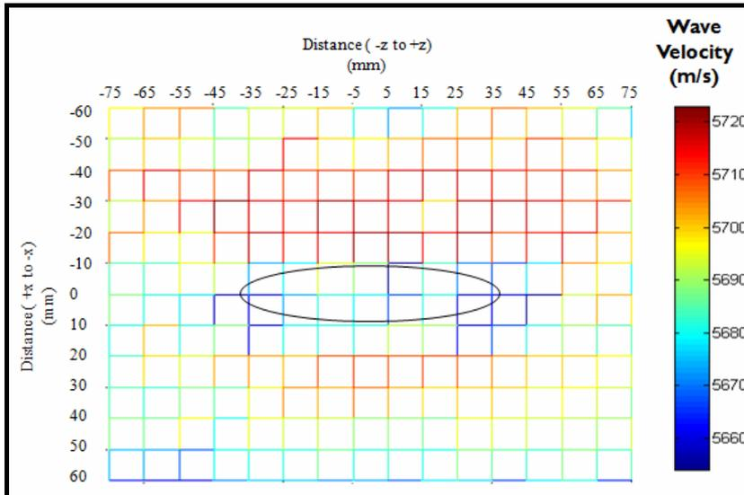
Figure 5. Ultrasonic wave velocity distribution in welded sample
