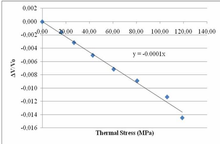
Figure 2.3. Relation between wave velocity change and thermal stress
