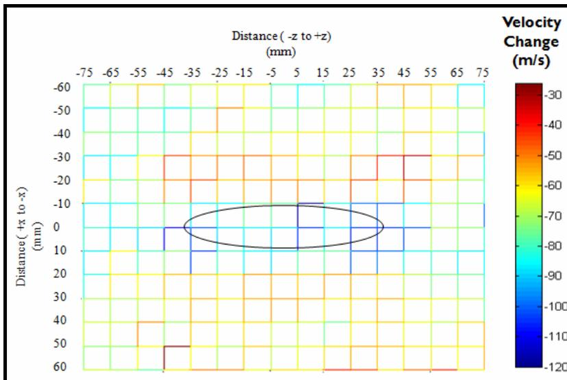
Figure 6. Ultrasonic wave velocity change after welding process
