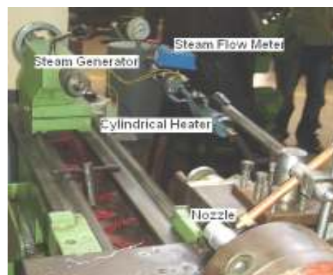
Figure 5. Steam generator and steam feeding system.
