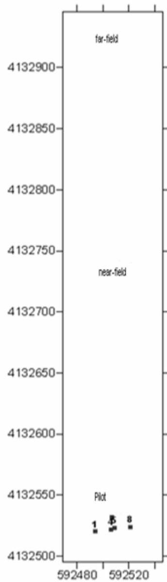
Figure 5. Experiment set to show the interaction between blast-holes: Far-Field: Far-field measurement station, Near-Field: Near-field measurement station. Pilot: Pilot blast. Distance between blast holes 4-5 is 3m. Distance between blast holes 1-8 is 21m.
