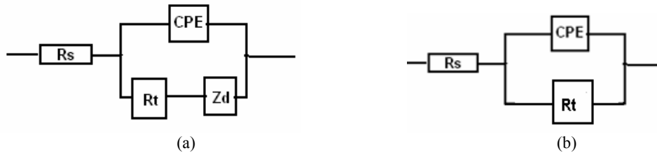
Figure 3. The equivalent circuit used to fit EIS data for copper displaying a Warburg impedance (a). The equivalent circuit used to fit EIS data for copper displaying a capacitive loop (b).
