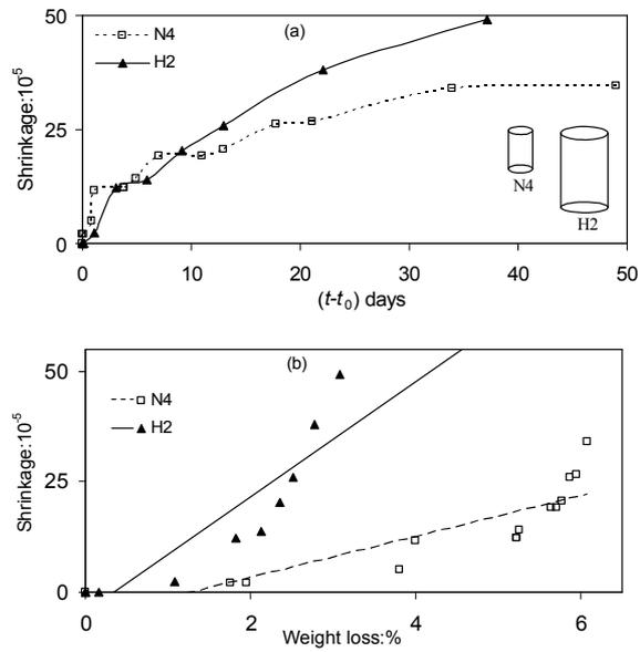
Figure 4. For HSC and normal strength cylinders, a) Effect of shrinkage, b) shrinkage-weight loss relationship.
