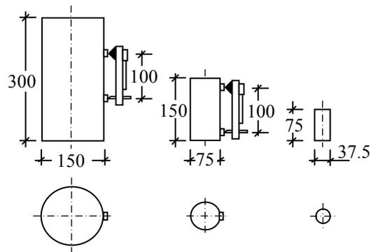
Figure 1. Test specimens for different sizes (mm).
