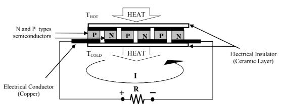
Figure 1. Thermoelectric module in generator mode
