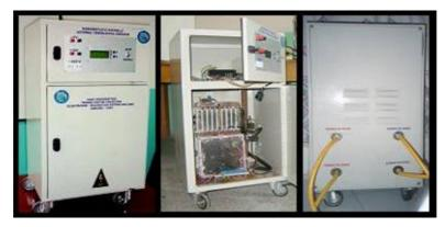
Figure 2. Microcontroller controlled geothermal thermoelectric generator
