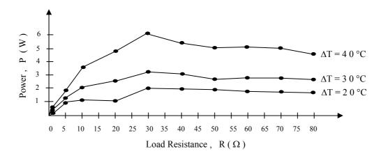
Figure 6. The Systems Load - Power relation
