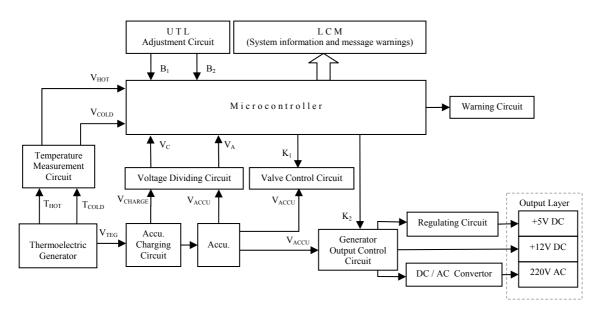
Figure 3. Block diagram of microcontroller based thermoelectric generator
