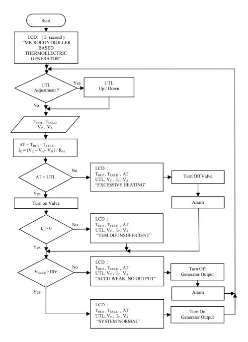
Figure 5. Flow diagram of microcontroller program
