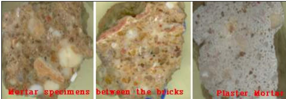
Figure 14. Mortar specimens, prepared for SEM and EDX analysis.
