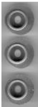
Figure 6. The manufactured cams using simple harmonic motion on the top, cycloidal motion on the middle and proposed cam profile on the bottom.
