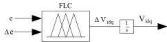
Figure 5. Structure of Fuzzy-PI controller.
