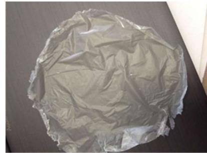
Figure 3. UHMWPE-HAp composite samples produced by gelation-crystallization method.
